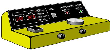
**Spectrophotometers** are used to measure the absorbance or transmittance of a liquid sample.
