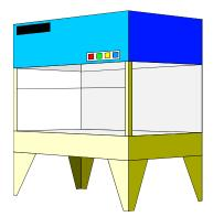
**Fume Hoods** are used to ventilate noxious or harmful gases.
