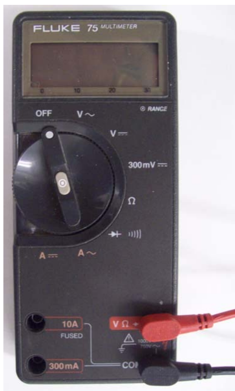
Figure 2. The Fluke 75 digital voltmeter used in this exercise to measure the potential.
