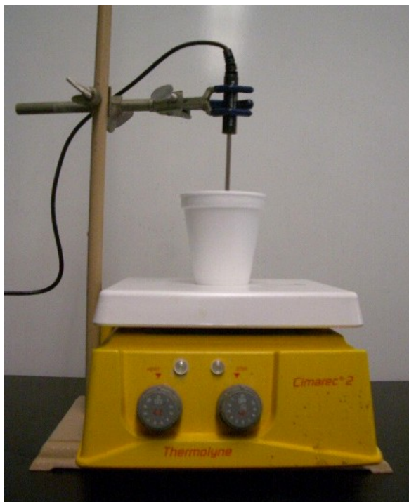
Figure 5. Experimental setup of the constant-pressure calorimeter (shown without the cover in place).
