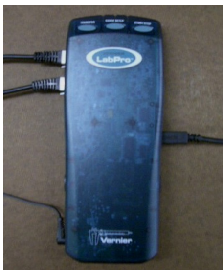
Figure 4. LabPro setup for this experiment showing temperature probes on both channel 1 and channel 2.
