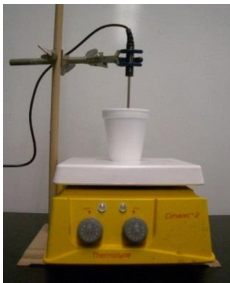
Figure 4. Experimental setup of the constant-pressure calorimeter (shown without the cover in place).
