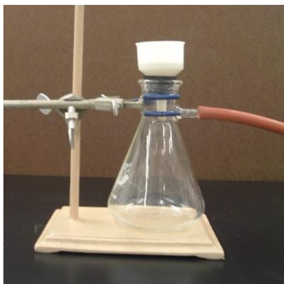
Figure 1. A properly configured vacuum filtration apparatus. Note the clamp that holds the filtration flask to the ring stand which prevents the filter flask from tipping over.
