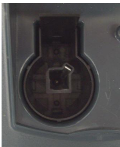
Figure 3. Enlarged view of the Genesys' sample compartment showing the sample holder. The light path is from the back of the instrument to the front (top to bottom in this view) as indicated by the arrow on the right side of the sample holder.
