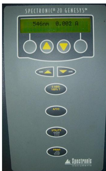
Figure 2. The Spectronic 20 Genesys control pad.
