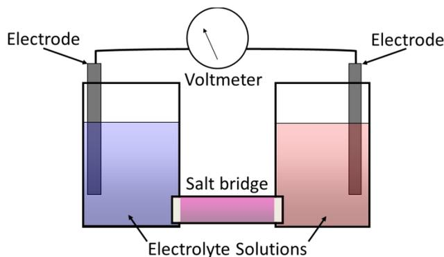
**Figure 1.** Schematic representation of an electrochemical cell.
