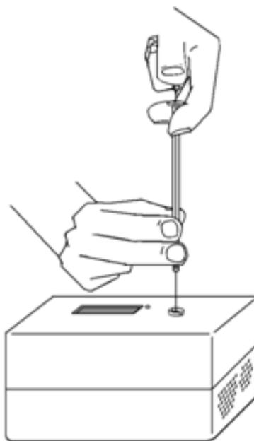
**Figure 2.** Proper method for injecting a sample into a Vernier Mini-GC.<sup>1</sup>
