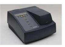
Your instructor may complete some of the steps below prior to the start of the lab period. Pay attention to your instructor's directions and do not press any keys on the spectrophotometer unless instructed to do so. Note: there are two arrow keys and two unlabeled keys below the LCD display. These keys are used to select or access alternate functions available on certain menus. Do not select these keys unless instructed to do so
